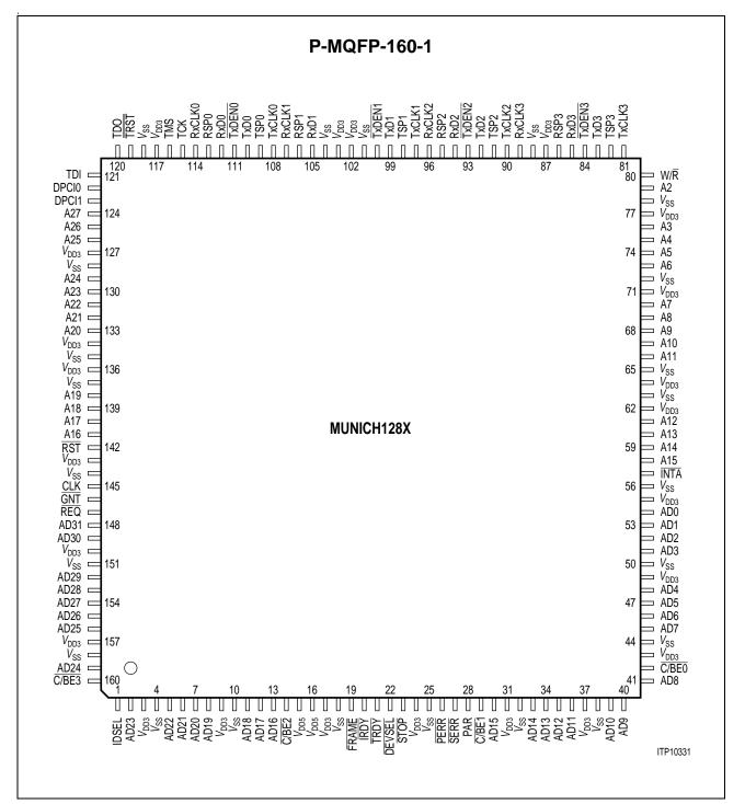
Figure 2-1 Pin Configuration
