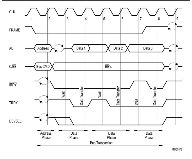
Figure 5-4 PCI Read Transaction
