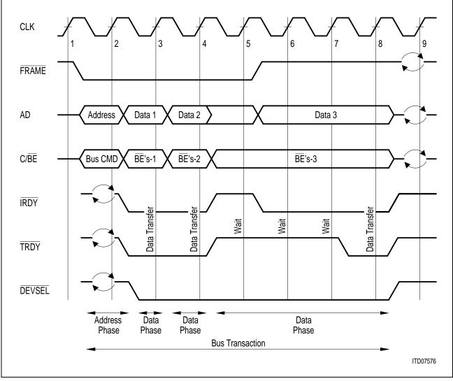
Figure 5-5 PCI Write Transaction
