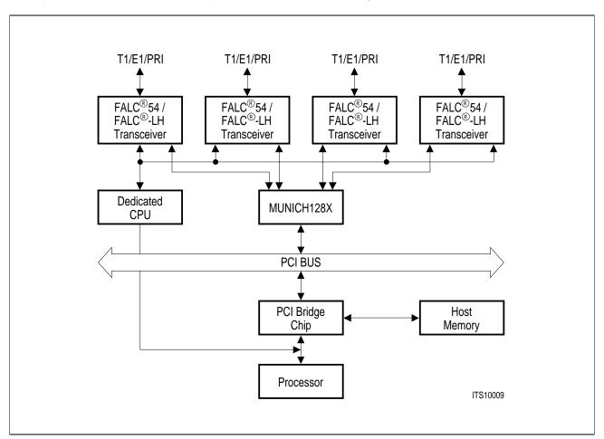
Figure 3-1 System Integration of the MUNICH128X in PCI-Based System
