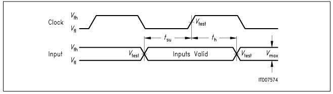
Figure 5-3 PCI Input Timing Measurement Waveforms
